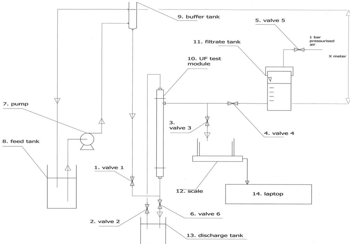
**Figure 1:** PID of the UF Pre-Test
