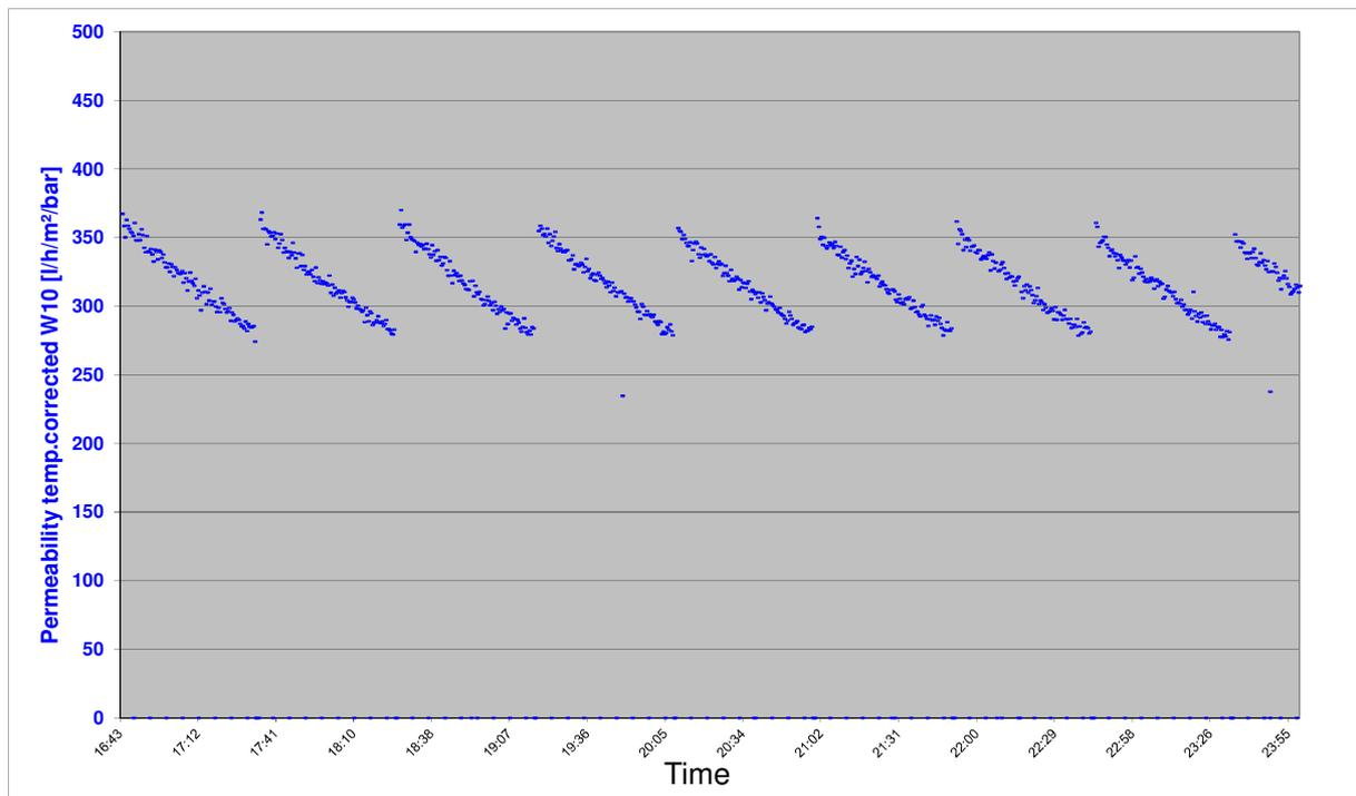
**Figure 3:** Part of a graph from a 75m<sup>2</sup> Liqui-Flux<sup>®</sup> W10 module for comparison; Wupper river water filtration at 89 l/h; backwash every 50 minutes
