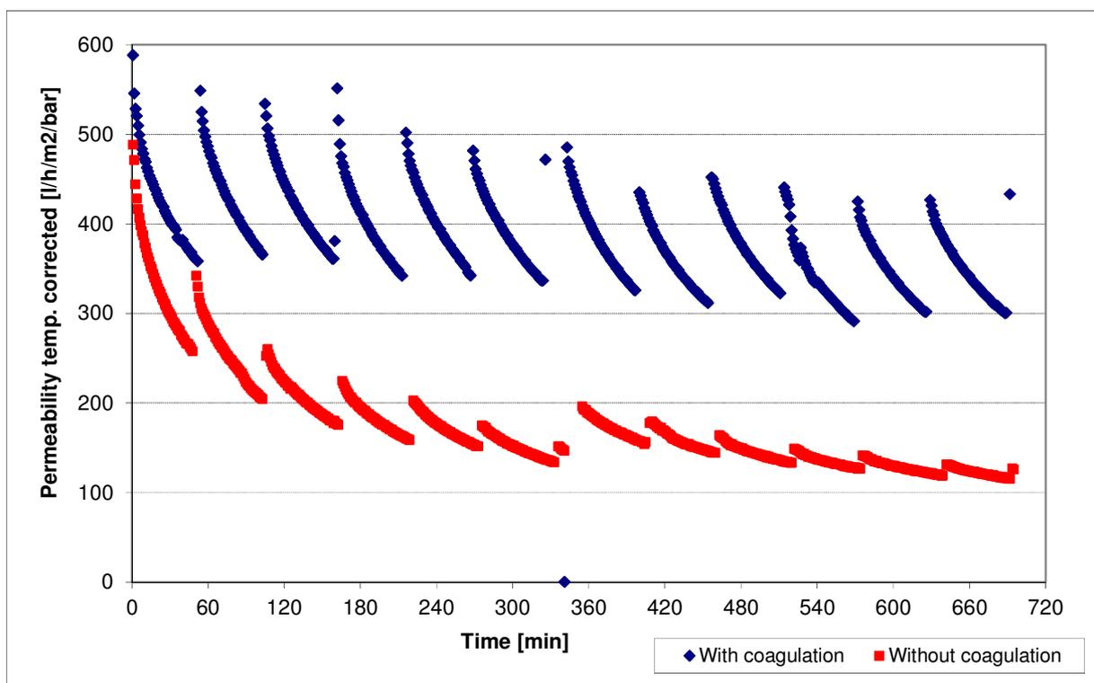
**Figure 4:** UF Pre-Test of river water (Wupper) with and without PACl coagulation (1000mm module length at 0.54 bar tmp)
