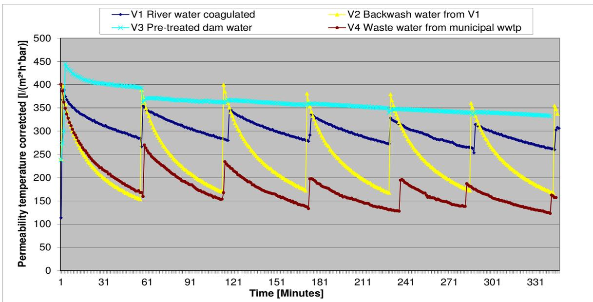
**Figure 2:** UF Pre-Test with different feed water qualities at a tmp of 0.3 bar; backwash @ 1bar
