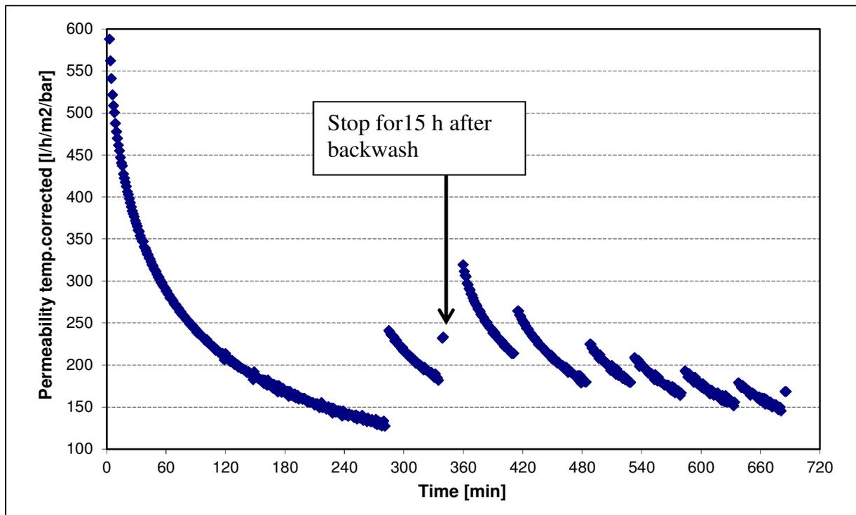
**Figure 6:** River water (Wupper); TMP=0.54 bar; module length=350mm; no coagulation; after 360 min. stop for 15 h
