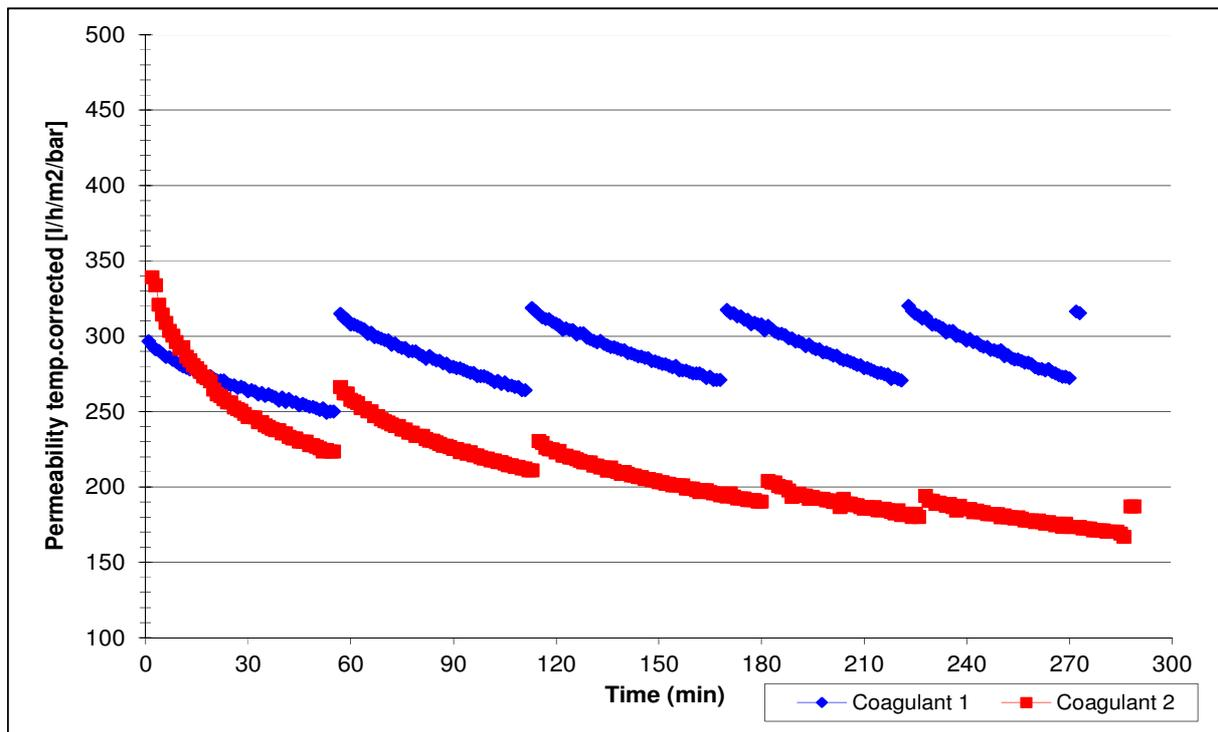
**Figure 5:** UF Pre-Test of well water with two different kind of PACl coagulation (1000mm module length and 0.54 bar tmp)
